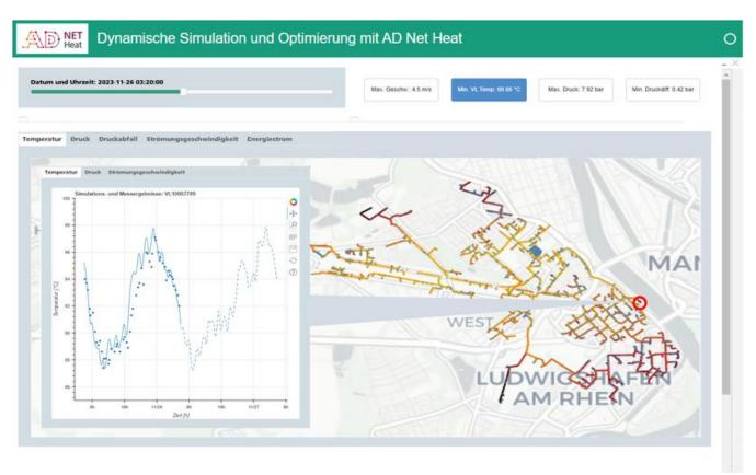
The graphical user interface displays the current temperature and pressure conditions in the network. © Fraunhofer ITWM
