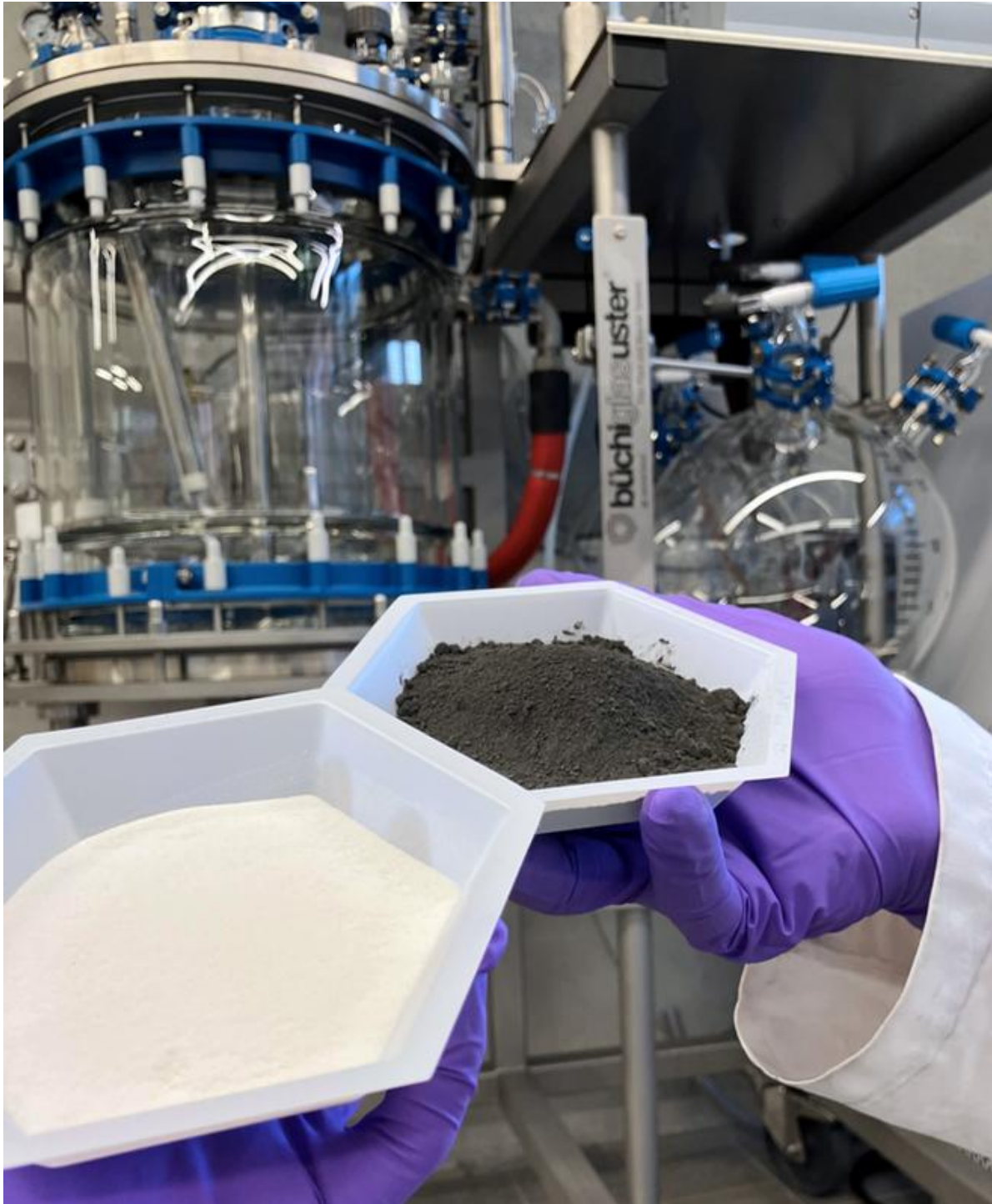
Lab-scale precipitation reactor for the development of an active material for sodium-ion batteries. © Fraunhofer IFAM
