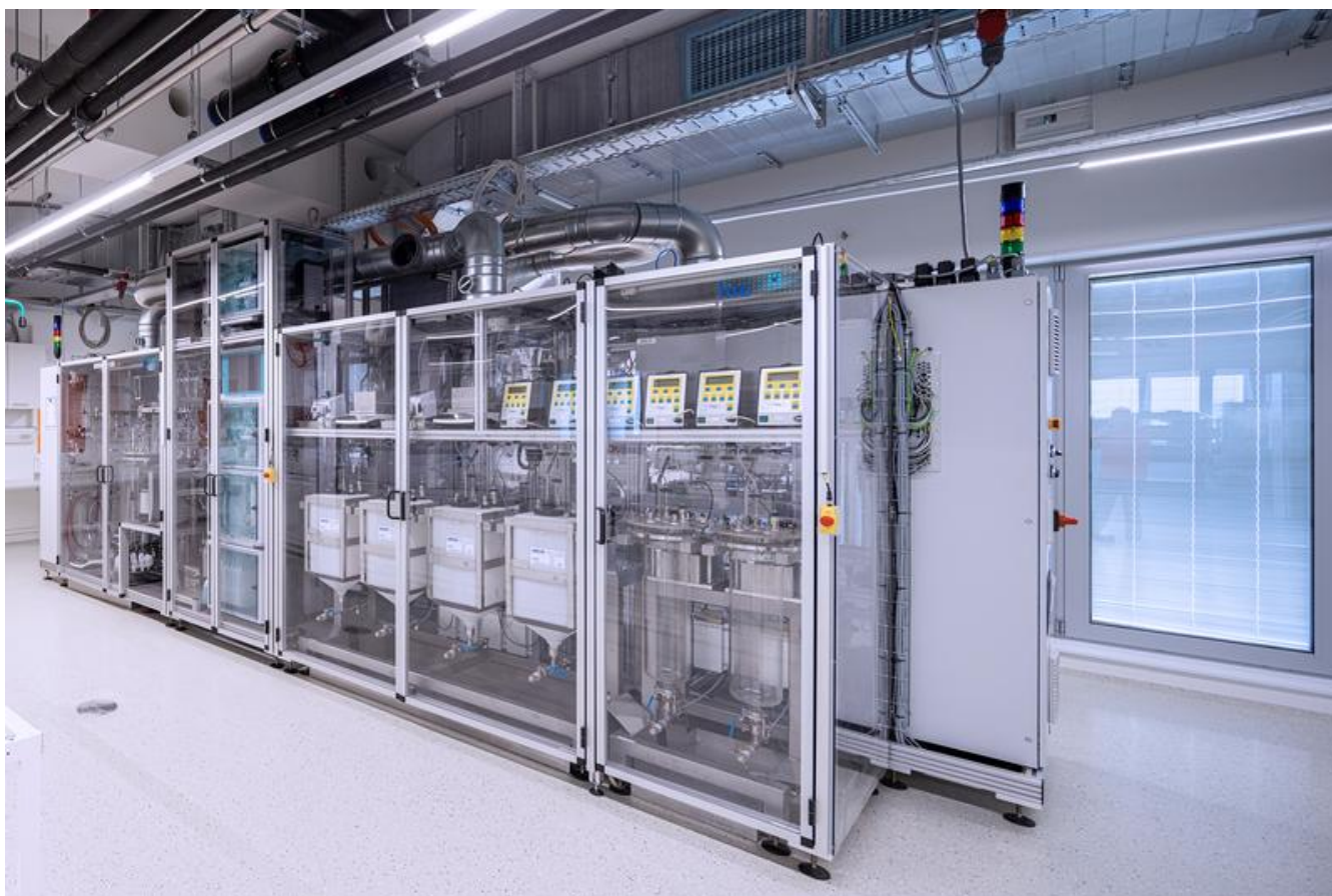
Powder-Up! Pilot plant for the production of active materials for sodium-ion batteries. © ZSW Ulm
