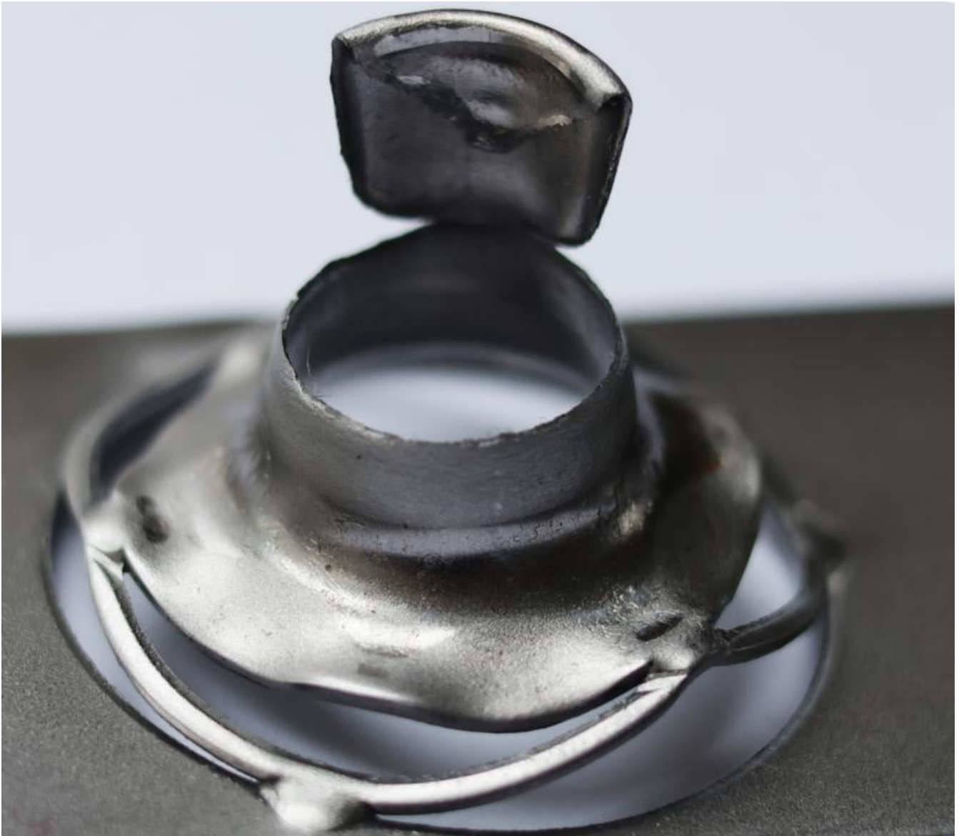
With identical parameters but without ultrasonic support, the metal cracks. © Fraunhofer IWU
