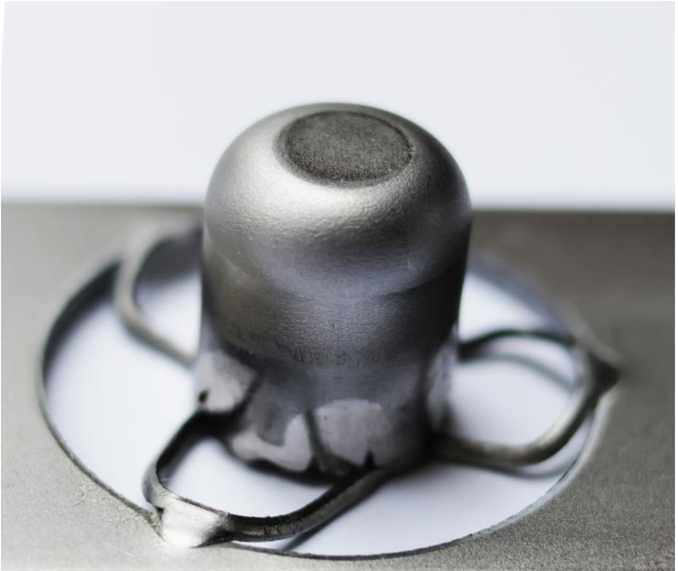
Ultrasonic deep drawing makes the difference: with a drawing ratio of 2.3 and vibration support, the deep-drawn ›bowl‹. © Fraunhofer IWU
