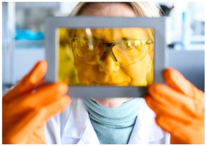
PFAS-free, catalyst-coated membranes are set to make electrolyzers and fuel cells significantly more environmentally friendly, cost-effective and powerful in the future. © Fraunhofer IAP, Jadwiga Galties
