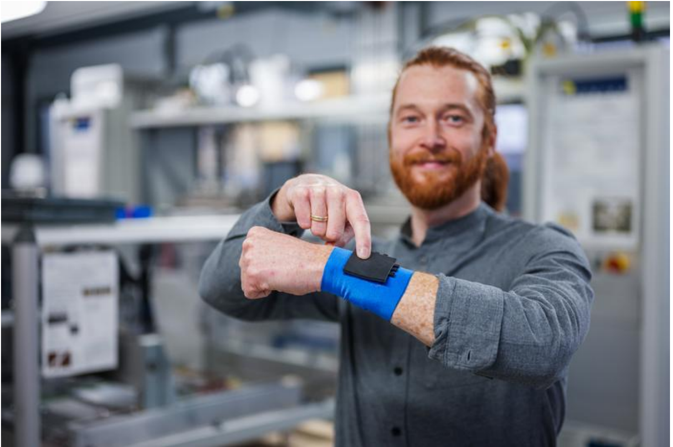
Researcher Sebastian Gratz-Kelly shows off a sensor element created from a metal-coated elastomeric film. The touchpad, here mounted on a wristband, can recognize the pressure and direction of a finger that swipes over it. Credit: Oliver Dietze Saarland University
