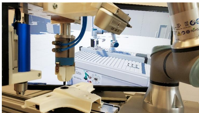
Fig. 2 GreenBotAI Demonstrator, Robotics made simple and efficient: Guided by 2D images, the robot picks up a component and inserts it into a second gear using intelligent, force-torque-controlled AI.
