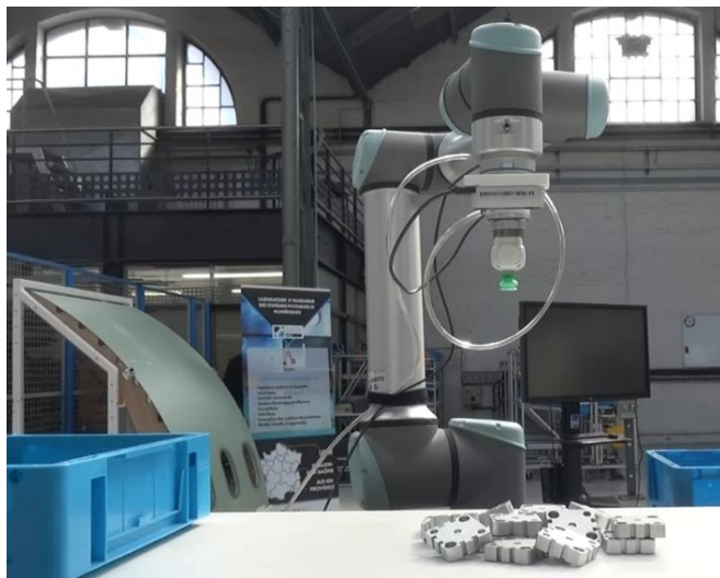
Fig. 3 GreenBotAI Demonstrator, Vision-Guided Robotic Picking made frugal and efficient: lightweight AI model is used to identify the position and orientation of the objects, and the robot trajectories are optimized. Energy consumption and picking time are reduced respectively by 30% and 8,5% as compared to conventional solution. ©ENSAM (Photo taken at Arts et Metiers Lille campus - LISPEN)
