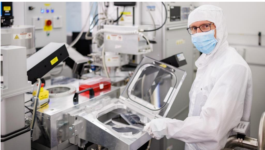
Researcher at Fraunhofer THM inserting a wafer into the transfer chamber of a deposition/etching cluster for structuring using atomic layer etching. © Daniel Karmann / Fraunhofer IISB
