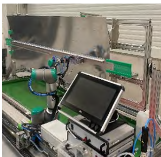
Figure 4 | Caption Anodizing station with robust component holder, precise linear axis and robotics, equipped with a specialized anodizing end effector for targeted, high-precision surface treatments (© Fraunhofer IFAM).
