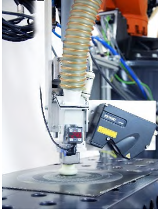
Figure 3 | Caption In addition to the robotic end effector including vacuum suction blasting nozzle, the developed vacuum suction blasting system includes a removal control sensor for inline monitoring for quality assurance (© Fraunhofer IFAM).
