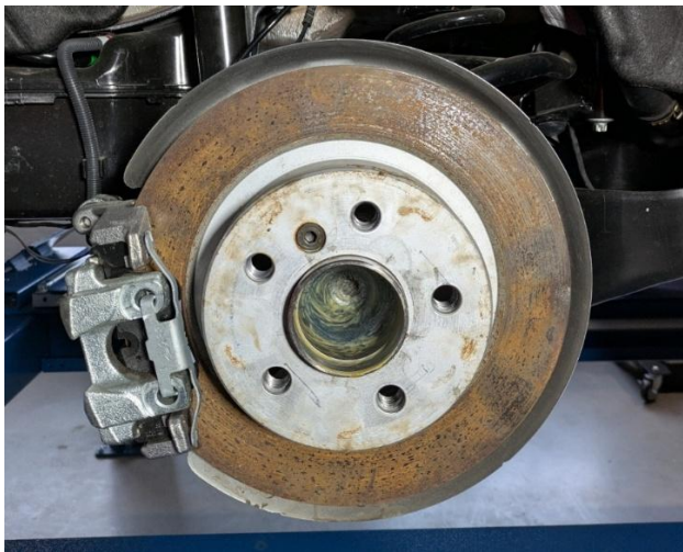
Fig. 2 Severe corrosion and scoring: gray cast iron brake disc that would no longer pass a mandatory vehicle inspection. Safe continued operation of the vehicle is no longer possible with this wear pattern on the brake disc. © Fraunhofer IWU
