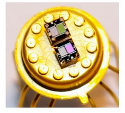
Picture caption: A gas sensor array developed by Fraunhofer IPM with four effective layers:  $SnO_2$ ,  $SnO_2/Pt$ ,  $WO_3$  and CTO. The dimensions of the sensor array are (1.5 x 1.5) mm<sup>2</sup>. (© Fraunhofer IPM)
