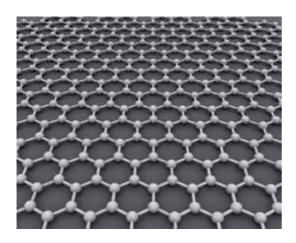
Graphene, which comes with up to 10 layers, is an expensive "all-rounder". It is not a natural resources that is found in the ground but must be manufactured. © Wikimedia.org /wikipedia
