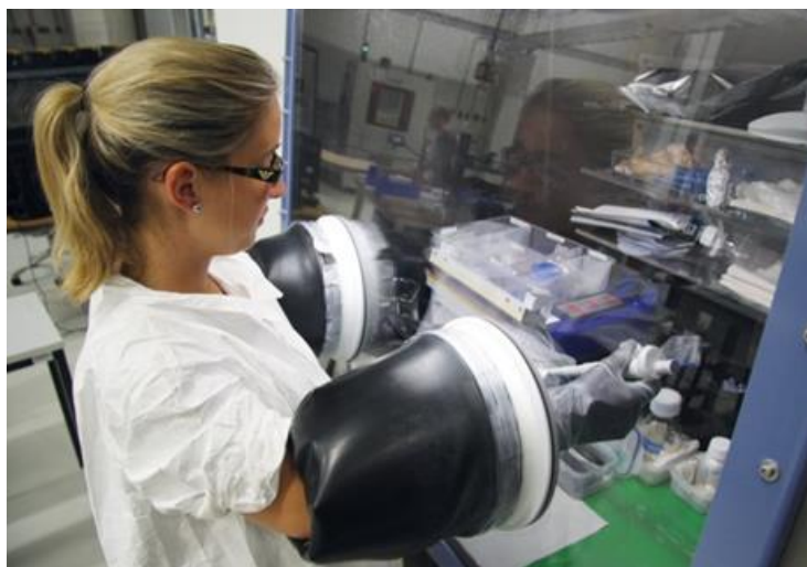
Employee working at a glove box at Fraunhofer ISE. She is filling electrolyte in lithium ion cells before formation. ©Fraunhofer ISE
