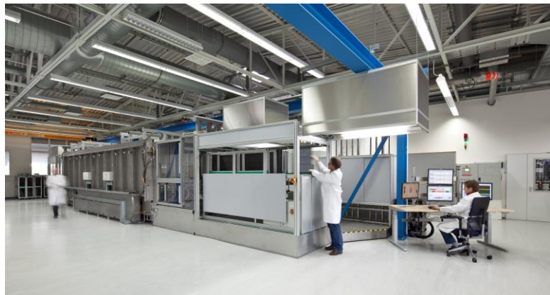
ProConCVD reactor for silicon deposition for epitaxial wafers. ©Fraunhofer ISE
