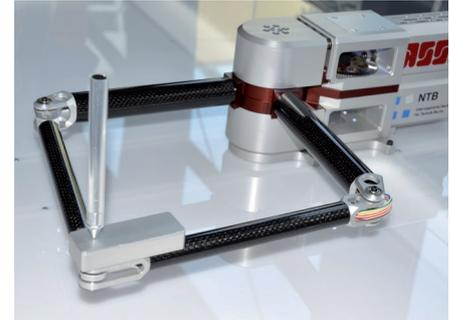
Stab balancierender Parallel-SCARA
