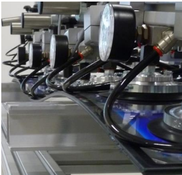
TPedge module with 2 mm thick glass undergoing distributed load test. ©Fraunhofer ISE
