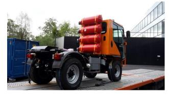
The electric drive LADOG vehicle with twelve 1 kWh battery modules shall reduce inner-city emissions caused by municipal vehicles. ©Fronius International GmbH
