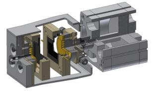
The test cell demonstrates homogenous operating conditions over the active area. The concentration, humidity and temperature gradients are negligible. ©Fraunhofer ISE
