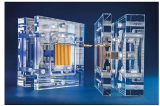
The test cell made of transparent plastic has been successfully implemented in research projects at Fraunhofer ISE for many years. In the photo one sees the current collectors, the gold-plated flow field plates and stamp. ©Fraunhofer ISE
