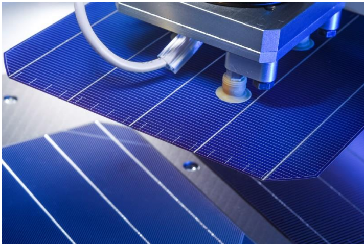
Solar cells with three, four or five busbars can be interconnected in the adhesive stringer. ©Fraunhofer ISE
