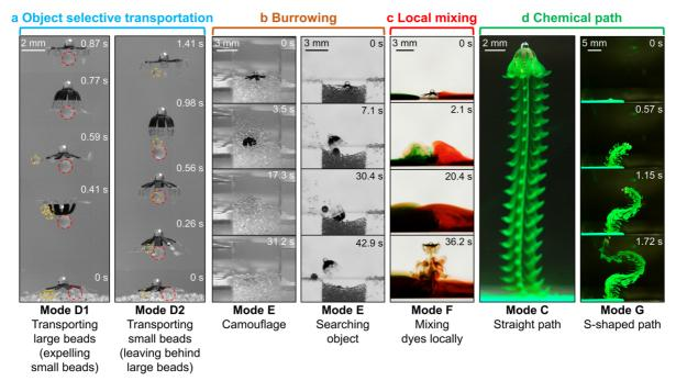
Figure 2. Four functions realized by the Jellyfishbot: a) transporting small and large beads; b) burrowing in a pool of fine beads simulating camouflage and search for prey; c) mixing two different colored food dyes; d) generating a chemical path.
