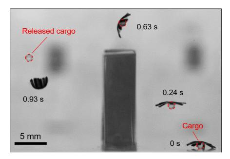
Figure 3. Cargo transport demonstration of the Jellyfishbot: The video snapshots of the robot and the bead are overlaid in the same video image. The red dashed circles indicate the positions of the bead being trapped and transported by the robot over a barrier.
