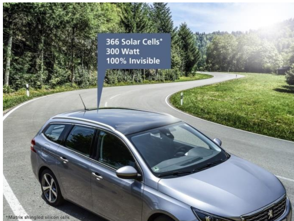
Photovoltaics integrated into a car roof: The Morpho-Color® coating of the glass cover allows the color to be adapted to the vehicle. © Fraunhofer ISE
