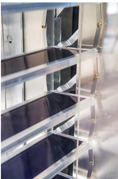
The slats of the solar thermal venetian blind (STVB) absorb the incident solar radiation. The heat is transferred to the collecting channel via heat pipes and an aluminum adapter. ©Fraunhofer ISE
