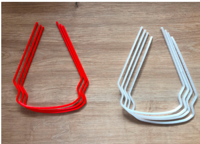
3D print sample of side pieces for safety goggles made from PLA and PC.
