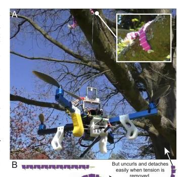
Fig. 1: A: Perching robot after suspending itself from a tree branch. Inset shows the compliant grapple passively wrapped around a branch. B: The compliant grapple passively curls to the shape of the branch, engaging the microspines to share the load, but still detaches easily.
