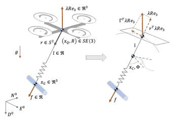
Fig. 2: The dynamics of the combined system  $(x_Q, x_G) \in \Re^6$  is decomposed into 3-DOF translation dynamics (7) of the center-of-mass of the system, the 2-DOF rotation motion (8) of the system around the CoM and the 1-DOF interaction dynamics (9). The quadrotor thrust vector  $\lambda Re_3 \in \Re^3$  is the control input to the system with  $\Gamma^T \lambda Re_3 \in \Re^2$  being the motion control component and  $r^T \lambda Re_3 \in \Re$  the force control component.
