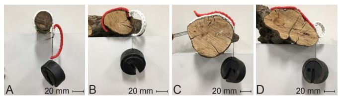
Fig. 3: Grapple shown suspending a 2kg payload from a variety of branch shapes, and conforming to irregular geometries.
