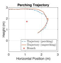
Fig. 6: Test showing the control fidelity during a perch/unperch manoeuvre. The actual position is recorded using a Vicon motion capture system. A: Demanded/actual tether angle. B: Resulting trajectory, with branch location indicated. The results show that the controller is functioning effectively, in spite of the unpredictable attachment of the grapple.
