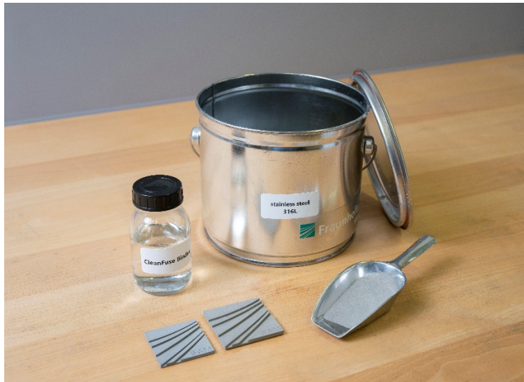
CleanFuse Binder, stainless steel metal powder and 3D printed parts before (right) and after (left) sintering. © Fraunhofer IFAM
