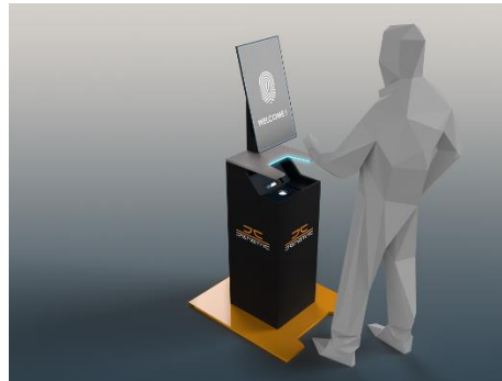
Fig. 2 and 3: "3D4F" makes it possible to capture fingerprints in a contactless and thus hygienically safe manner. © Jenetric
