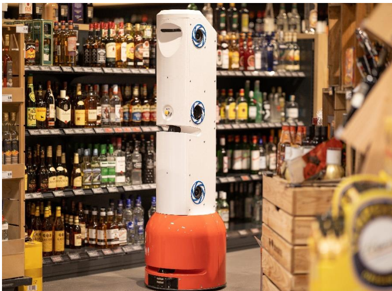
Fig. 4: By automatically recording stock levels, it eases the workload on retail staff - the service robot "TORY", developed in the joint project "ROTATOR".
