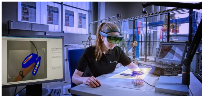
Fig. 2: Augmented reality assistance system used to support manual testing of components or large surfaces; © Uwe Bellhäuser
