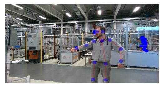
The "Robo-Dashcam" records safety-relevant data and persons in compliance with data protection regulations while the robot cell is in operation. This means that the safety concept can still be adapted at a later date. Image credit: Fraunhofer IPA
