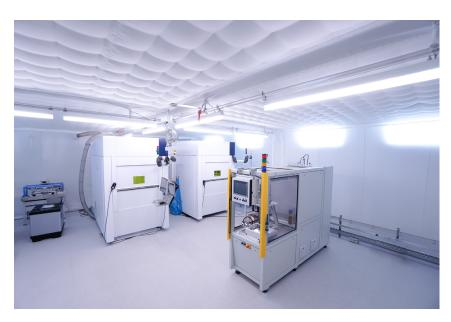
The dry cleanroom system DryClean-CAPE® not only creates a clean production environment, but also one with very low humidity.
