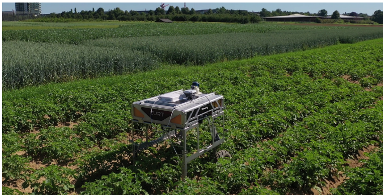
The large robot CURTdiff can autonomously recognize and move along rows of crops, for example. In this way, it could potentially be used for weed control in future. Source: Fraunhofer IPA
