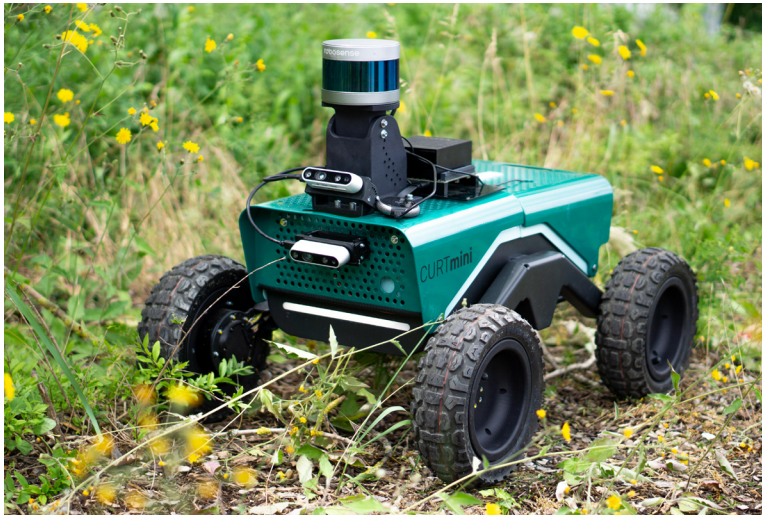
The small, mobile robot CURTmini autonomously recognizes different ground types, assesses these in terms of traversability and accordingly plans a suitable route. Source: Fraunhofer IPA
