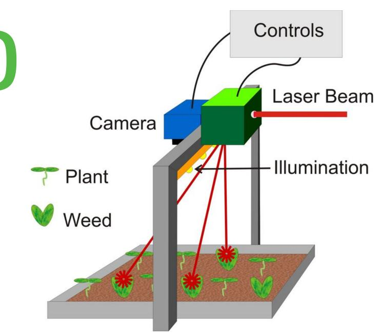
orking sketch of the laboratory set-up for weed control using the laser. Image processing recognizes which plants are which, and aims the laser only at the weeds.
