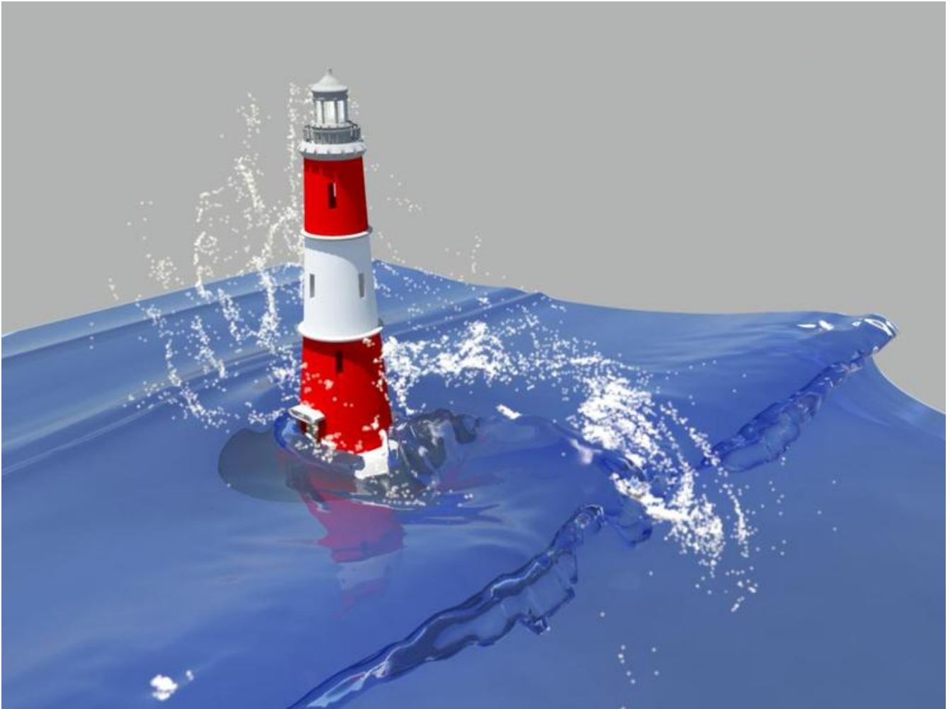
Two-phase fluid flow with coupled particle droplets © M. Griebel, P. Zaspel (Institute for Numerical Simulation, University of Bonn)
