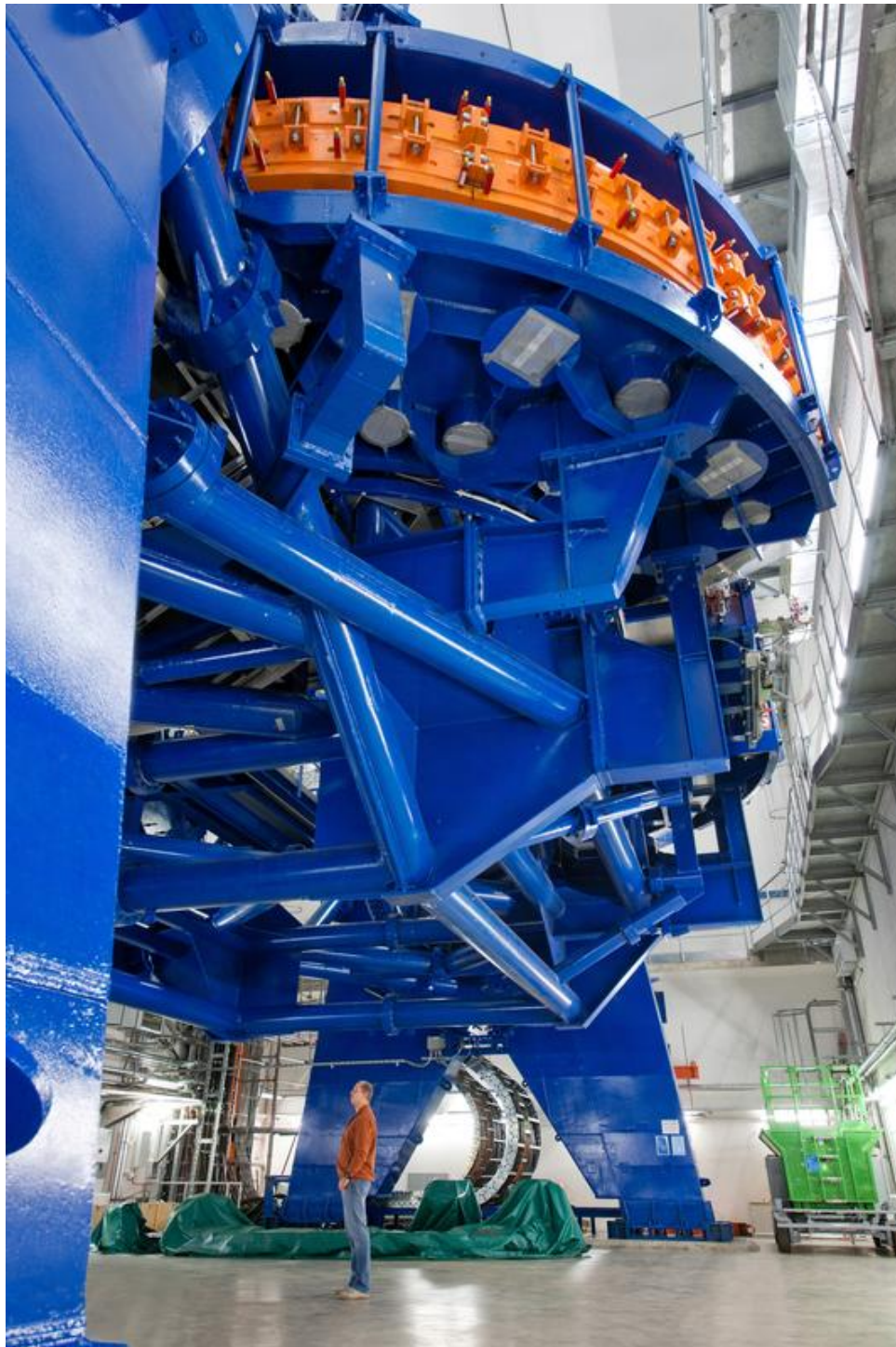
The gantry at the Heidelberg Ion Beam Therapy Center (HIT) is a 360° rotating beam delivery system for heavy ions. The world's only such facility, the gantry is a gigantic steel construction weighing 670 tons. It is 25 meters long, 13 meters in diameter and spans three stories. Photo: Heidelberg University Hospital
