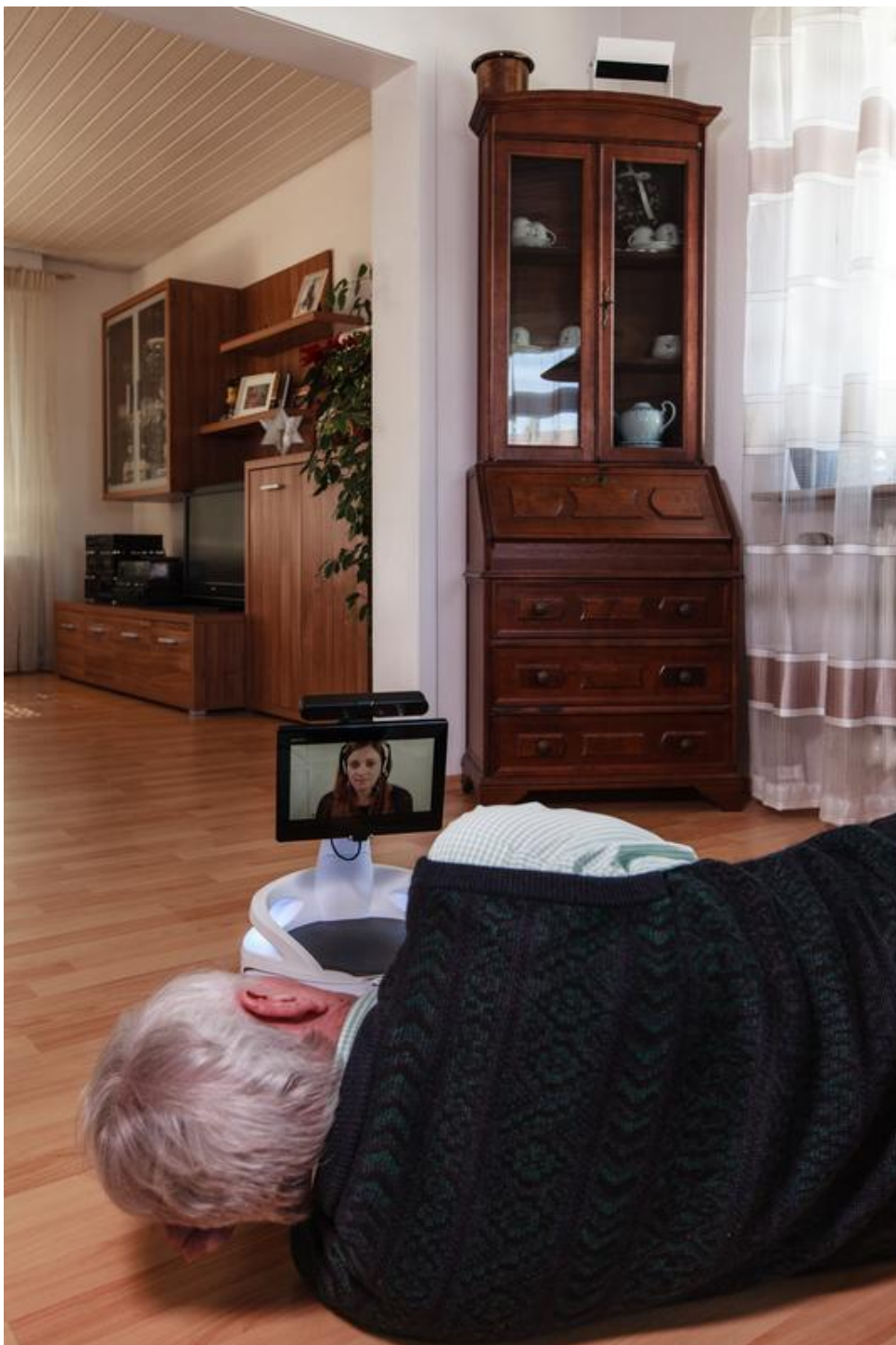
The sensor-system for fall detection can be placed up on high furniture or it will be mounted on the ceiling. The robot serves as a mobile communication system. Fraunhofer IPA
