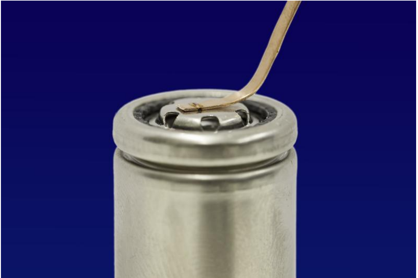
Oscillation laser welding creates safe electrical contacts between battery cells. Picture source: Fraunhofer ILT, Aachen/Germany.
