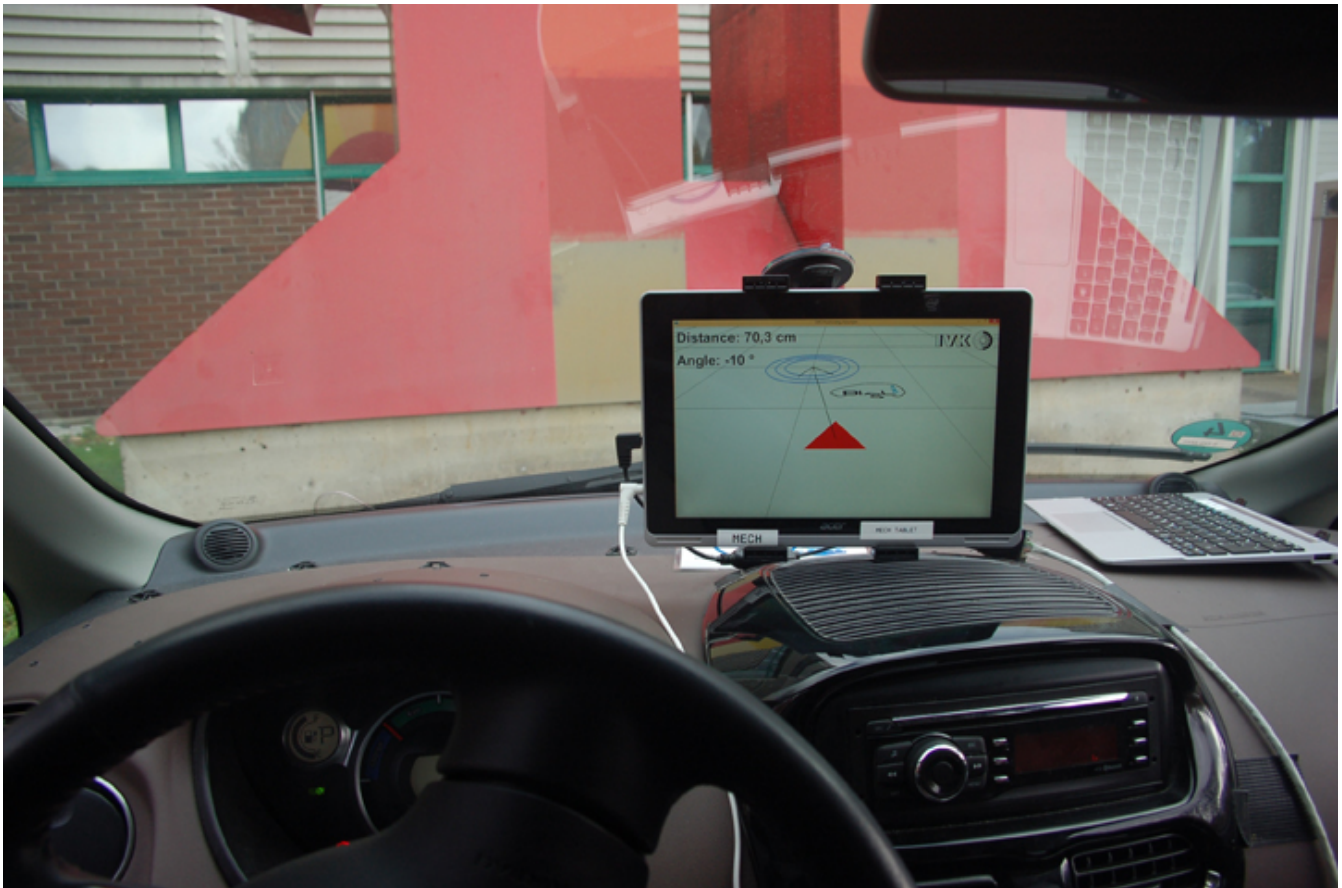
3D display of the position of the charging coil (receiver coil red, charging coil blue) University of Stuttgart / IVK
