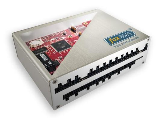
Central control unit of foxBMS, the free, open, and flexible battery management system from Fraunhofer IISB in Erlangen.
