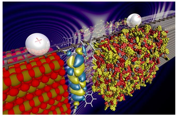
Visualization of a current through an OLED, flowing via a thin molecular layer (center) from an electrode (left) to an organic semiconductor (right).
