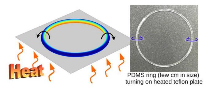
With the wheel within, the researchers hit upon an extremely simple principle to set polymer materials into spontaneous motion.
