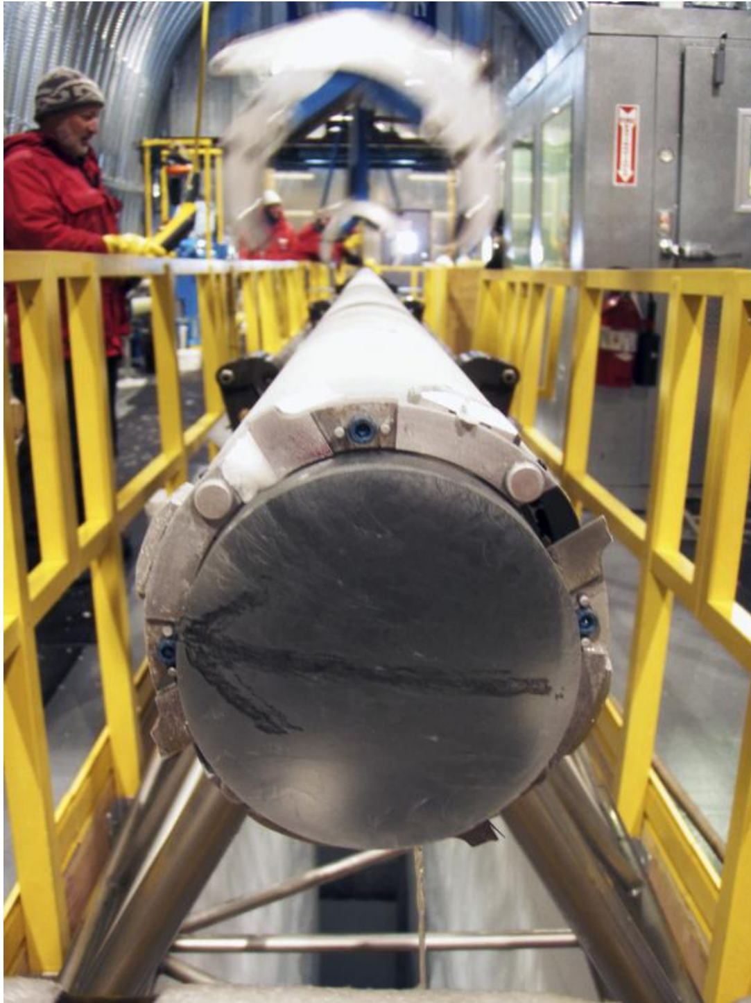
Freshly drilled segment of the WAIS Divide ice core is brought to the surface. Photograph courtesy of Tommy Cox
