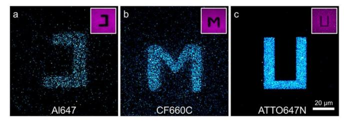
Three dyes used for fluorescence microscopy. The carborhodamine dye (r.) shows more efficient photoblueing than the two cyanine dyes. Team Markus Sauer University of Würzburg
