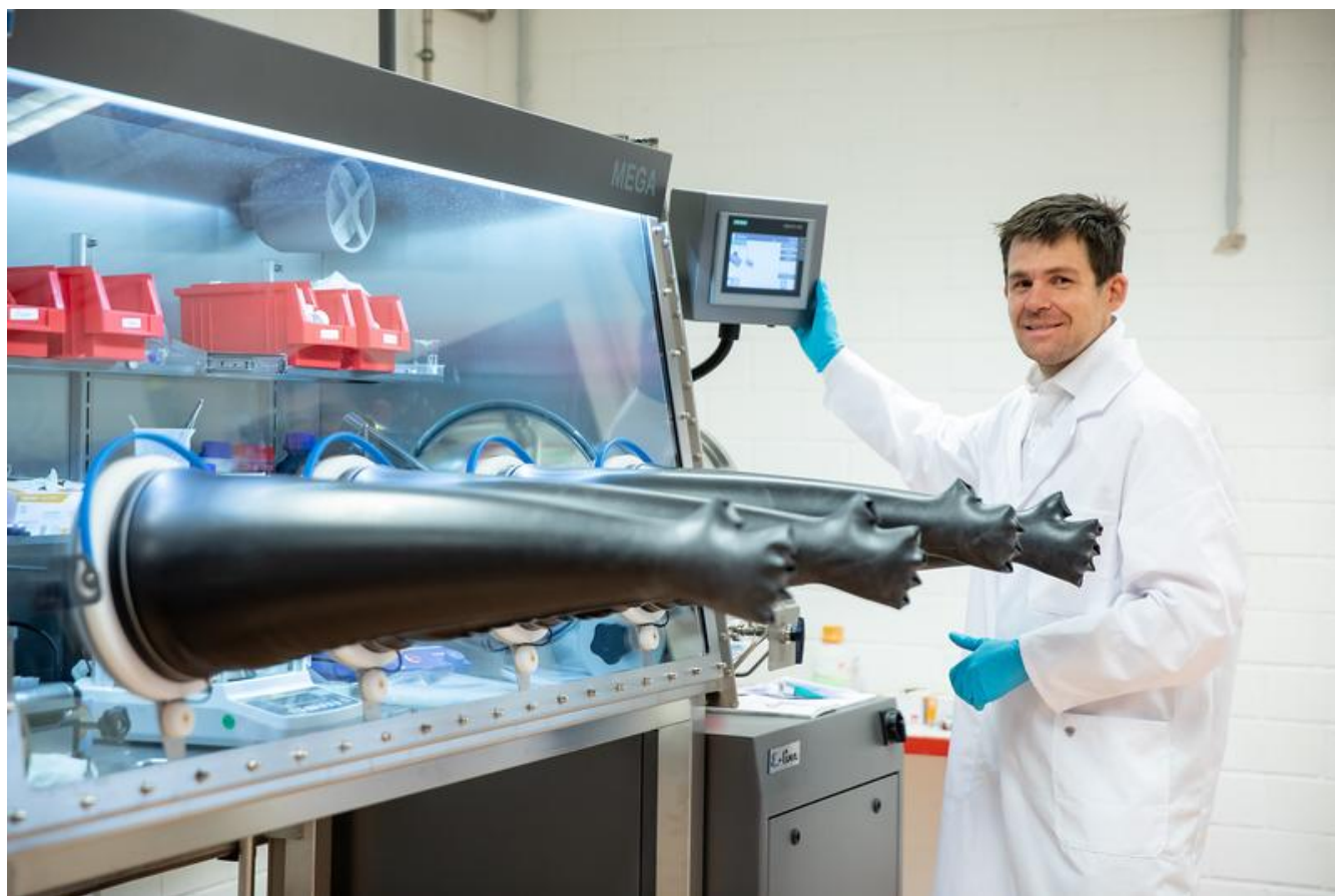
Prof. Oliver Clemens on a glove-box, in which air-sensitive samples can be safely processed and stored. Uli Regenscheit Universität Stuttgart
