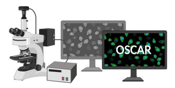
OSCAR (optical stem cell activity reporter) can be used to detect dormant stem cells in tissue. A short peptide is incorporated into the backbone of a fluorescent protein. Due to the lack of phosphorylation, an increase in green fluorescence is observed.
