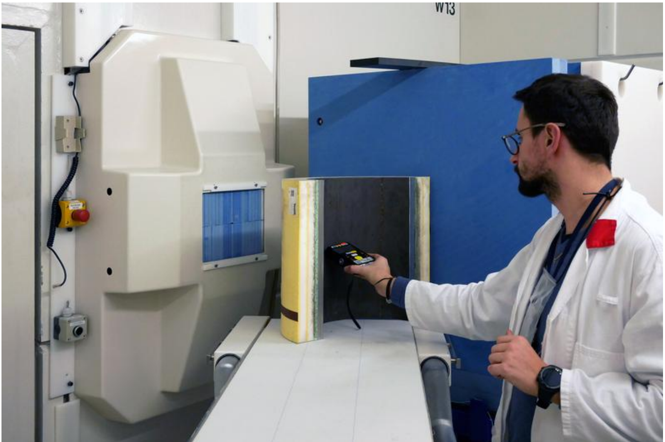
Zeljko Ilic adjusting a pipe segment for one of the neutron experiments at the instrument FANGAS.
