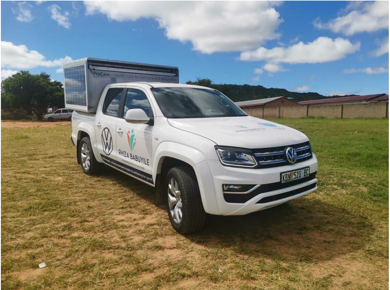
The first prototype of the care unit mounted on a Volkswagen Amarok. Frank Neumann © Fraunhofer IST
