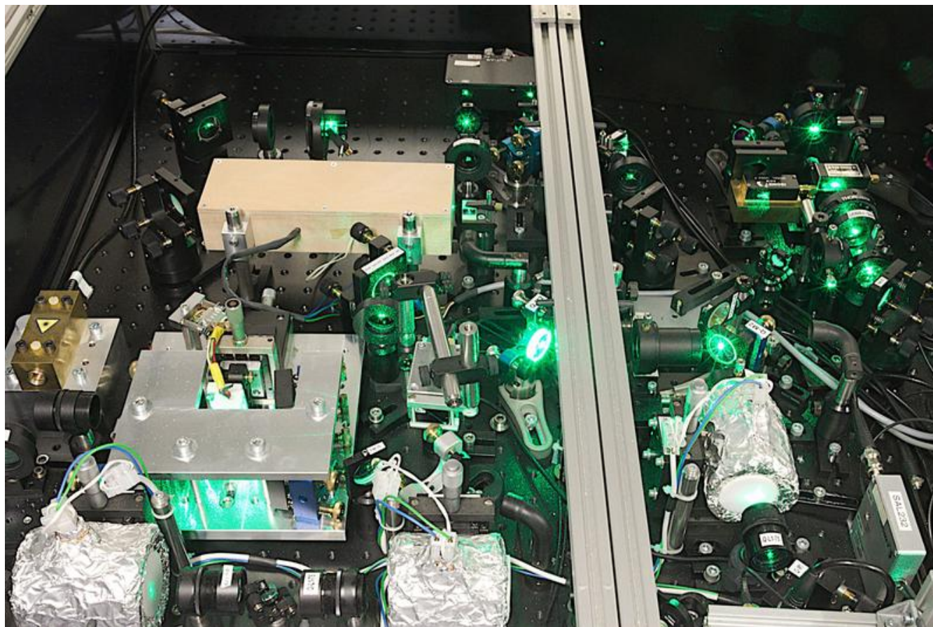
Macroscopic trial set-up for complex laser systems in an optical atomic clock.
