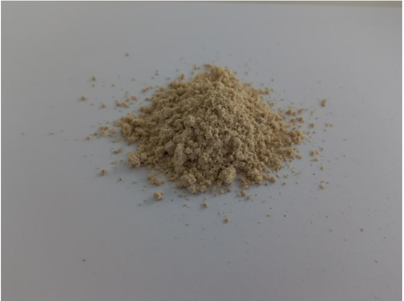
The rapeseed concentrate obtained from the EthaNa ® pilot plant contains over 40 percent high-quality proteins. Fraunhofer CBP
