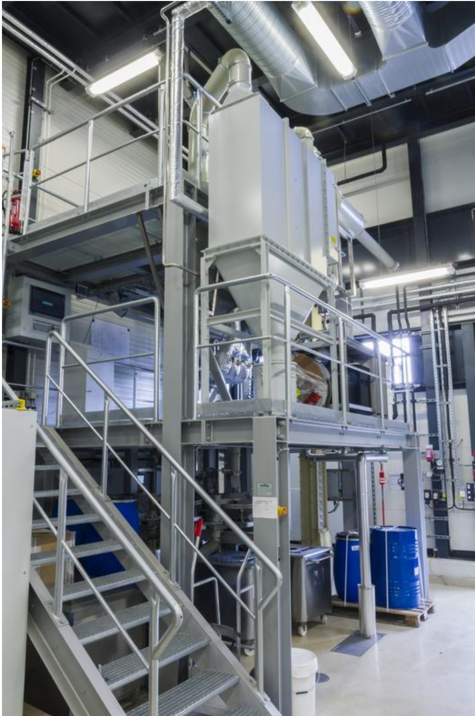
In the de-hulling plant, up to 100 kilograms of rapeseed per hour can be de-hulled in continuous operation. Fraunhofer CBP
