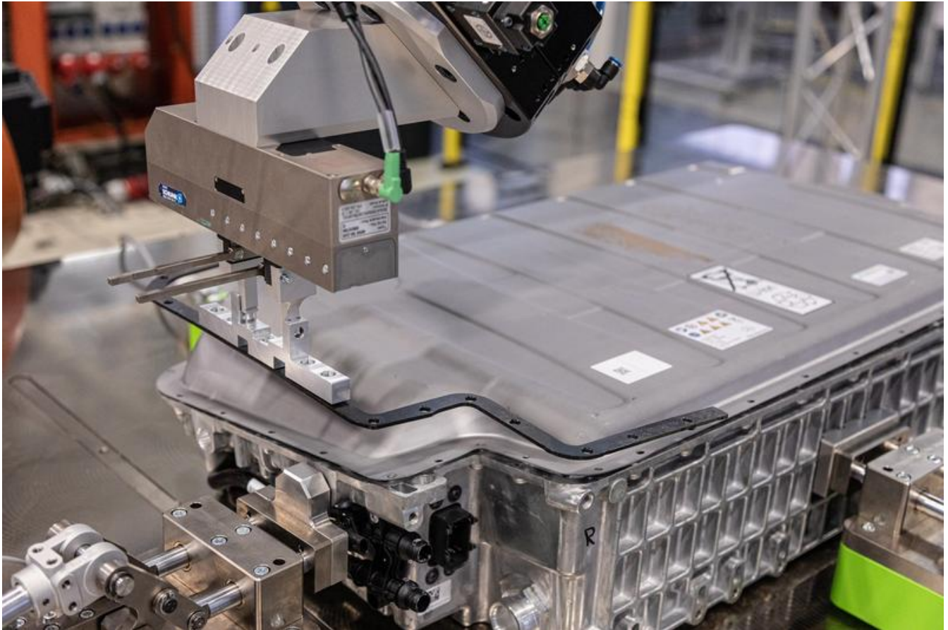
The project developed a variety of hardware for automated disassembly tasks, such as this small parts gripper. Rainer Bez Fraunhofer IPA
