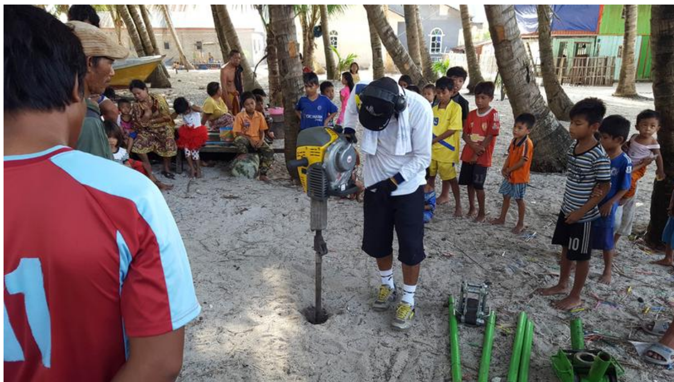
Taking a drill core on the coral island of Barrang Lompo. Dominik Kneer
