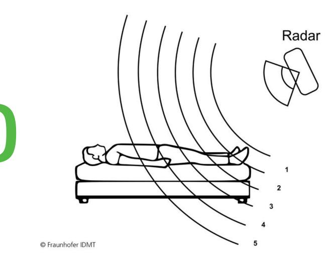
By positioning the radar from the side, the researchers at Fraunhofer IDMT can collect vital data from the various areas of the body particularly clearly, such as respiratory parameters on the torso and the heartbeat pulse on the legs. Fraunhofer IDMT Fraunhofer IDMT
