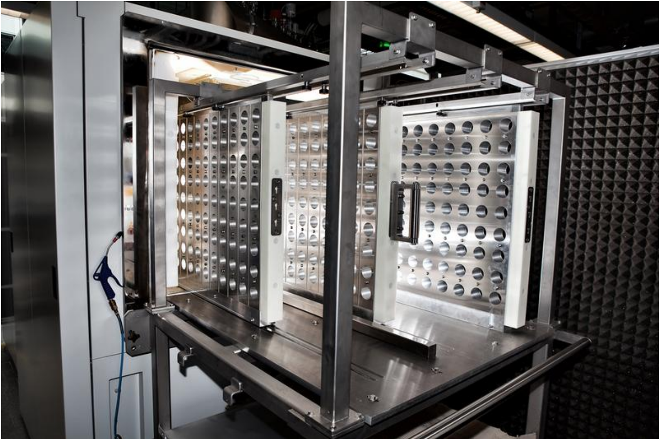
Low-pressure plasma system with easily exchangeable electrode systems, which also function as product carriers. © Fraunhofer IFAM
