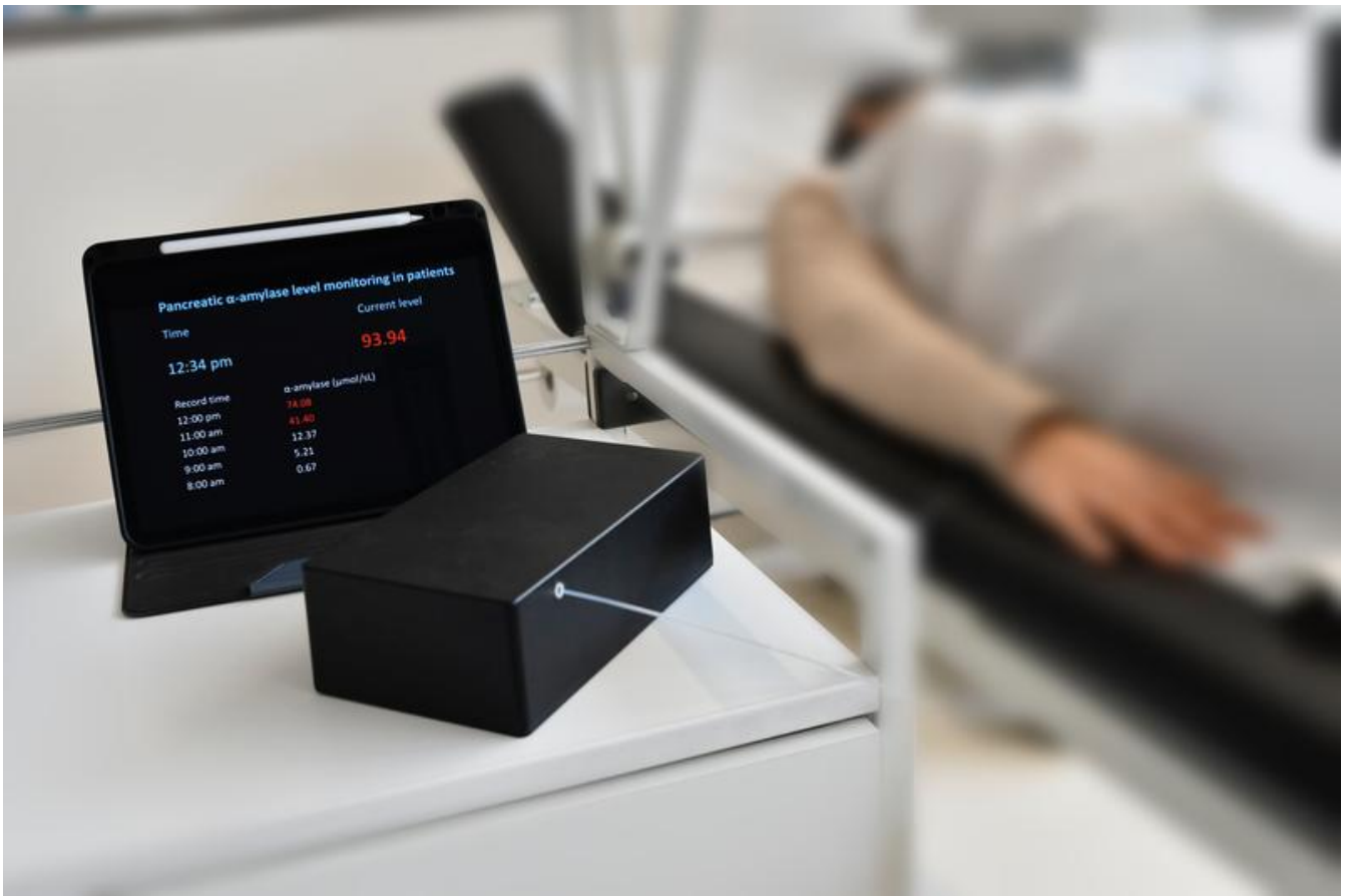
The Millifluidik device is positioned next to the patient's bed and enables real-time monitoring of amylase activity. Xinne Zhao HZDR / Xinne Zhao
