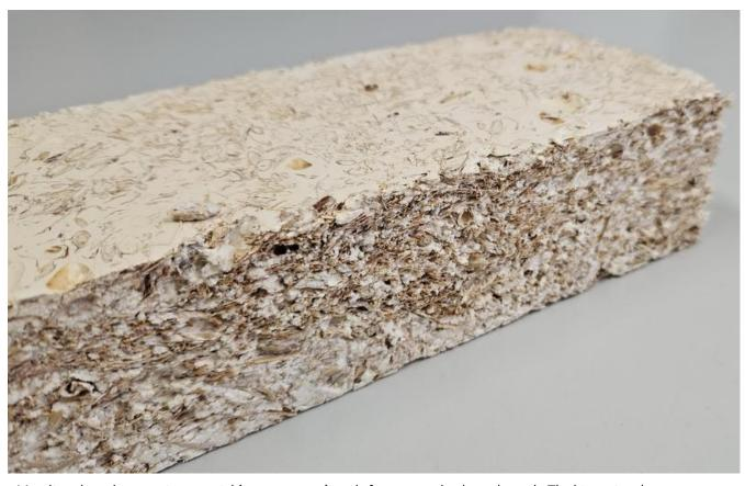
Mycelium-based composite material ( $25 \times 9 \times 5.5$  cm) made from straw, husks and starch. The biogenic substrate was 3-dimensionally intergrown and bound by the mycelium of the fungus Ganoderma resinaceum and the composite was then heat-dried and sanded.
