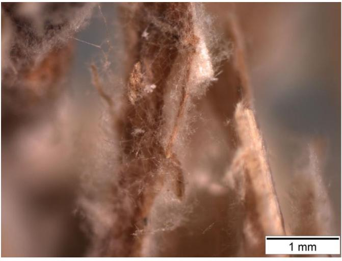
Mycelium of the fungus Ganoderma resinaceum on a natural substrate consisting of loosely packed straw particles with an average length of 2 cm, which were previously broken down using a hammer mill. (Image: Binocular) Michael Unger University of Göttingen/Michael Unger
